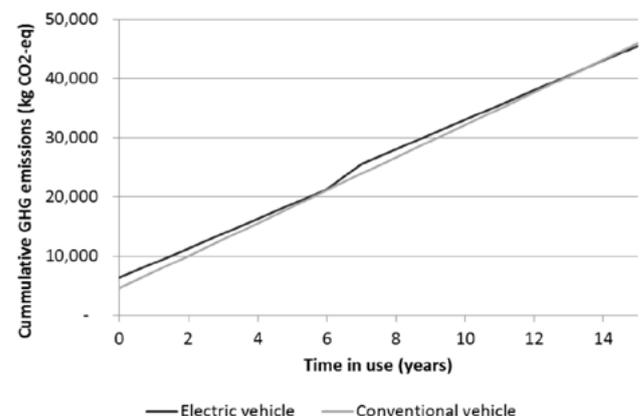
**Figure 1: Comparison of the cumulative GHG emissions of an electric vehicle and a conventional vehicle used in Australia.**
